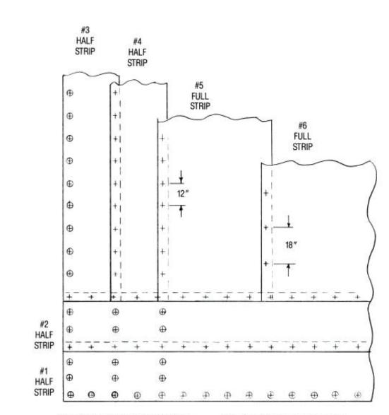
TOP FASTENERS WITH REINFORCED OUTPOST FASTENER COVERS (SHOW AS ⊕)
