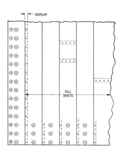
ENDS OF SHEETS ARE LAPPED 4½" TO ALLOW FOR FASTENING AND WELDING. FASTENERS ARE INSTALLED ON 12" CENTERS, FLUSH WITH BOTTOM EDGE. ALTERNATE PERIMETER FASTENING WHERE HALF-STRIPS ARE NOT USED IS SHOWN. TOP FASTENERS WITH FASTENER COVERS PLACED IN CENTER OF STRIPS AS INDICATED. FASTENERS GENERALLY PLACED ON 12" CENTERS FOR THE FIRST SIX FEET OF STRIPS FROM EDGE. (SHOWN AS  $\oplus$ )
