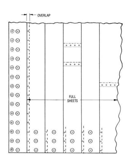
ENDS OF SHEETS ARE LAPPED 4½" TO ALLOW FOR FASTENING AND WELDING. FASTENERS ARE INSTALLED ON 12" CENTERS, FLUSH WITH BOTTOM EDGE. ALTERNATE PERIMETER FASTENING WHERE HALF-STRIPS ARE NOT USED IS SHOWN. TOP FASTENERS WITH FASTENER COVERS PLACED IN CENTER OF STRIPS AS INDICATED. FASTENERS GENERALLY PLACED ON 12" CENTERS FOR THE FIRST SIX FEET OF STRIPS FROM EDGE. (SHOWN AS  $\oplus$ )
