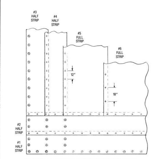
TOP FASTENERS WITH REINFORCED FLEXION FASTENER COVERS (SHOW AS )
